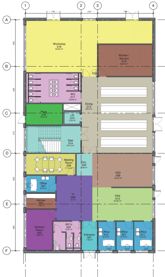
Ground Floor Plan - Initial GA Plan Proposal Scale 1:100
