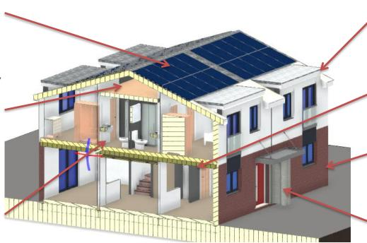
Super insulated, air tight and thermal bridge free envelope reduces demand for heat
